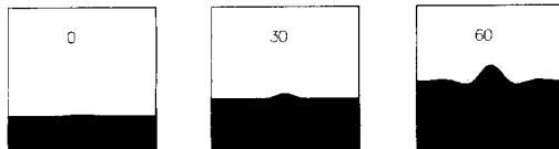
FIG. 4. Dendrite convergence study. Physical parameters: \varepsilon_C = \varepsilon_V = 0.02 , A = 0.5 , k_A = 4 . Numerical parameters: J = 40 , N = 60 , t = 0, 0.75, 1.5 .
